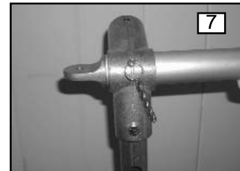
Custom PTE installed and pinned into a PTI at the right side of the inside radius
